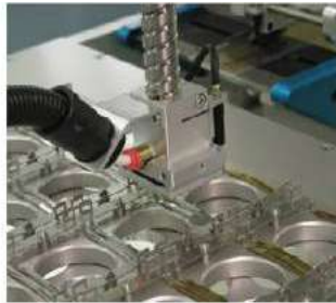
Placing of an insulator onto a fan clip.
