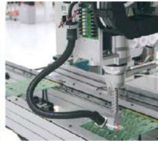
Assembly of adhesive backed dome switch arrays onto a PCB. PCB shows very high tolerance.
